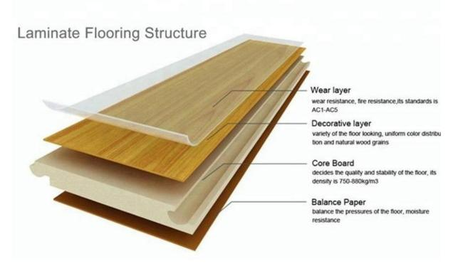
Wear Layer: Laminate flooring is a surface layer of two thin sheets of paper infused with melamine. A protective wear layer to provide hardness and protection. This top-most surface layer is a hard transparent type of plastic sheet that is impervious to dogs, chairs, high heels, and other common damaging elements. This layer is extremely tough, making laminate one of the most durable flooring options around.
