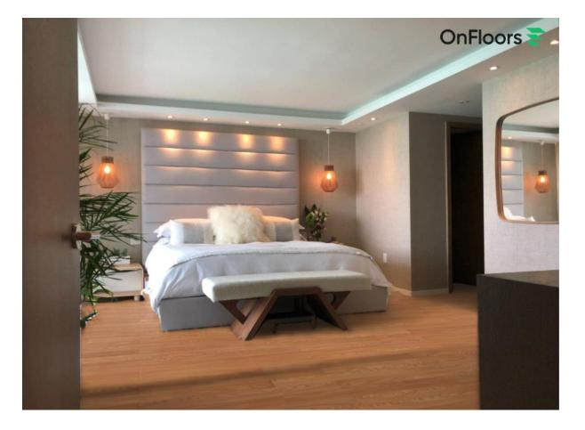
Laminate floors are a hybrid floor covering consisting of a particleboard wood base topped by an image layer and a transparent wear layer. Simply put, laminate is a hardwood floor alternative. It's extremely popular thanks to its attractive price point and the fact that it can mimic just about every type of wood flooring you can imagine (some like stones too).
