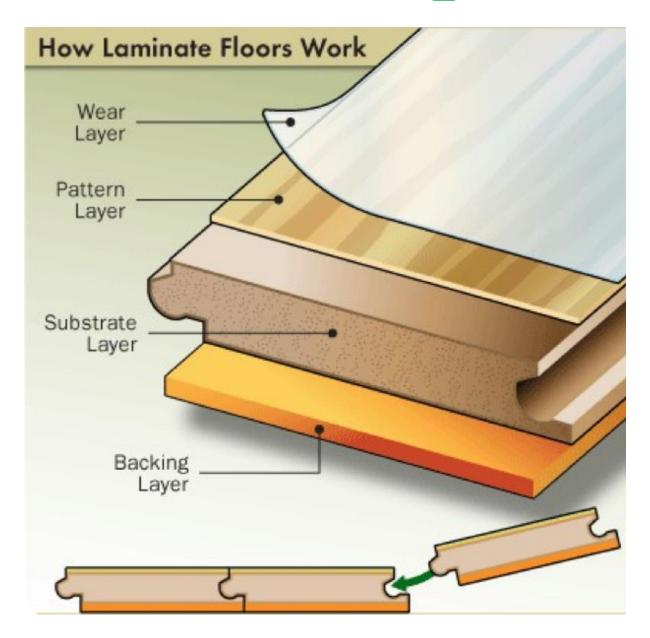
**HDF Core Layer:** Under the wood-grain photograph is about a half-inch of woodchip amalgamated. to give the material strength and stability. This base is the same one used in many of the best engineered wood flooring products
