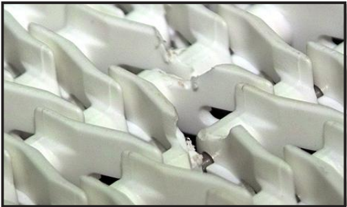
Inspect Chain for broken links
