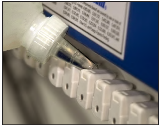
Lubricate the conveyor wearstrip with silicone oil
