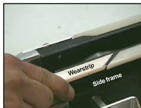
Figure 14: Slide wearstrip into side frame
